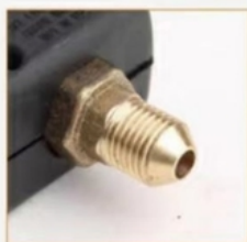
280/380管接头 (14*1.5mm螺纹)
