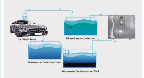
**Purification Process Schematic Diagram**
